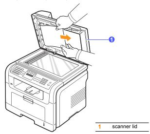
Close the scanner lid. Then load the removed pages back into the ADF.
